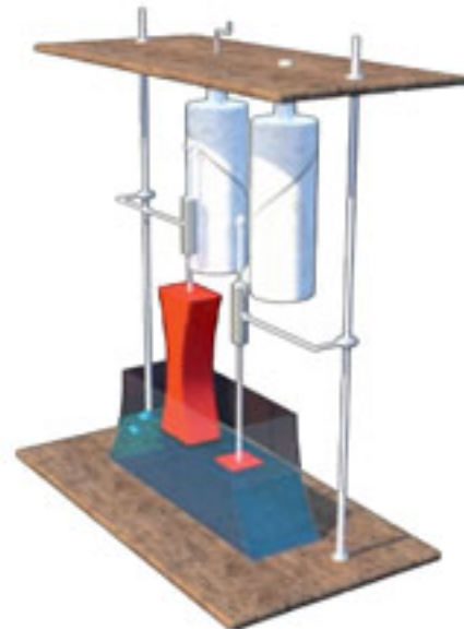
Figure 3. 3D model of basic elements of a hydrointegrator with a rotating input roller, author of 3D model Petar Vranić (Mathematical Institute of SASA)
