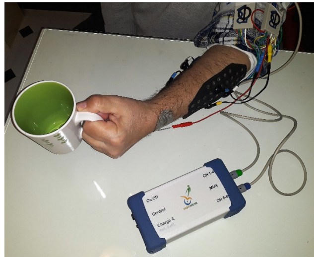
Figure 3: Image of the MOTIMOVE and the MAGNETRODE with all required wiring for the FET of the grasping.
