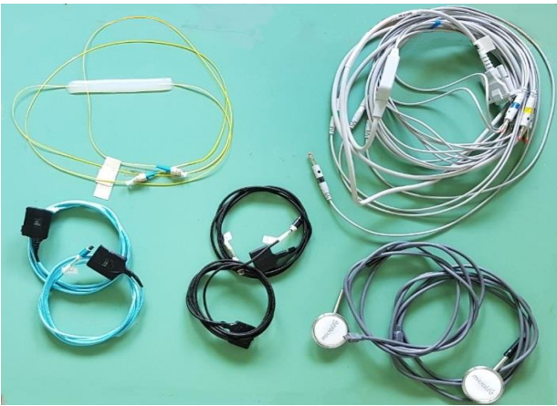
Figure 3: Different sensors used in measurement - fiber optical sensor (up left), ECG electrode cable (up right), photoplethysmography sensor (bottom left), accelerometers (bottom center), digital stethoscope (bottom right)
