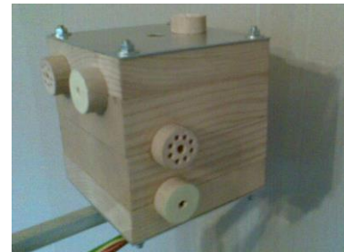
Figure 1a. Three-axis' heat loss anemometer (prototype) in thermally insulating (wooden) housing comprises NTC thick-film segmented thermistors: actual size 100 · 100 · 100 mm.
