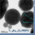
Nanostructures with crystallite size around 20 nm are in good agreement with XRD refinement.
