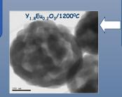
Rougher particle surface evident in the thermally treated samples corresponds to larger primary crystallite size
