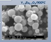
Thermally treated samples show that the spherical particle morphology is maintained throughout the thermal treatment and that the higher temperature regime provokes further crystallization and growth of primary particles.
