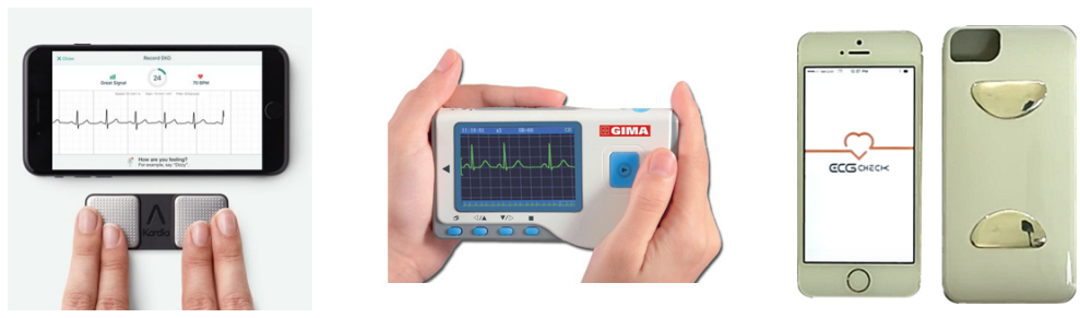
Fig. 1. Examples of the hand-held ECG devices on the market: Kardia, AliveCor, US (left panel); CARDIO-B PALM ECG, GIMA, IT (middle panel), ECG check, Cardiac Designs, US (right panel). All three devices use stainless steel electrodes.
