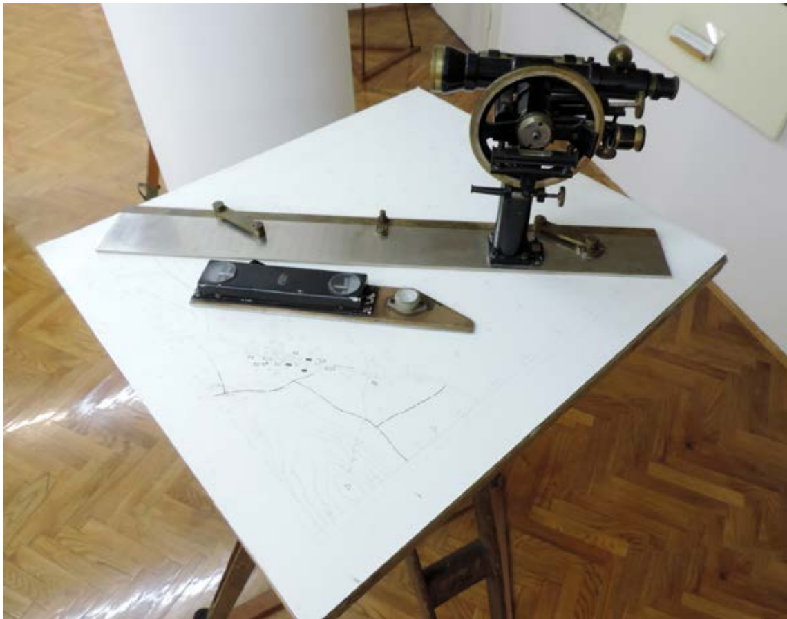
Fig. 3. Plane table with telescopic alidade or kipregel (Military Geographical Institute, Belgrade; photo: Z. Vuksanović-Macura)
