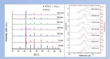
Mechanical activation leads to the creation of new surfaces and decrease in particle size of the initial powder particles, which affects the crystallization of PVDF matrix. In addition, prolonged mechanical activation leads to agglomeration of nanoparticles agglomerates of different sizes.
