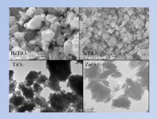
Microstructural changes due to mechanical activation in ZnO, BaTiO<sub>3</sub>, SrTiO<sub>3</sub> and TiO<sub>2</sub> powders were investigated using electron microscopy (TEM and SEM), x-ray diffraction (XRD) and particle size analysis (PSA). These were correlated with molecular simulations of mechanical properties of PVDF-nanocluster composites with different oxide nanocluster sizes (1, 1.5 and 2 nm)
