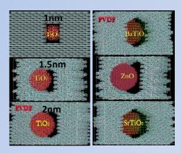
Each system was simulated using a periodic system of metal oxide nanocrystal inside  $\beta$ -PVDF matrix.  $\beta$ -PVDF was chosen for its superior properties over  $\alpha$ - and  $\gamma$ - phases. Geometry of each system was optimized prior to the calculation of mechanical properties using GULP v4.3 software package.
