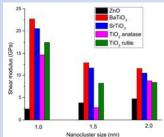
Molecular simulations show that, in general, mechanical properties (Young modulus as an indication of elasticity, Shear modulus as an indication of hardness) for all systems improve with decrease in nanocluster size. This suggests that mechanical activation of fillers in PVDF-metal oxide nanoparticle composites should have a positive effect on the mechanical properties of composite systems.
