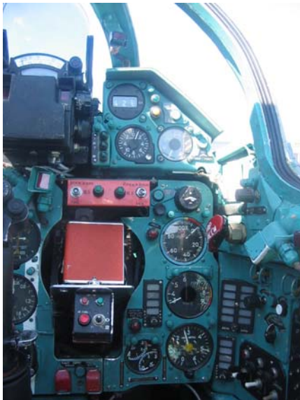
Picture 1. An example of integration of photo recorder in the cockpit of L-17 fighter
