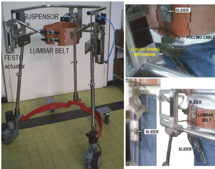
Fig. 6 – The prototype of the modular hip orthosis fitted into the Walkaround ® developed for Tecnalia Inspiring Business, San Sebastian, Spain.
