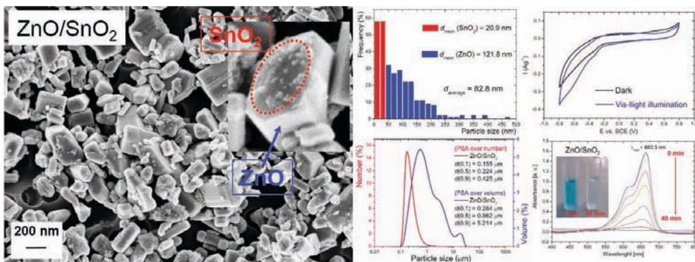
**Figure 1.** FE-SEM micrograph, particle size distributions, and photo(electro)catalytic activities of ZnO/SnO<sub>2</sub> composite.
