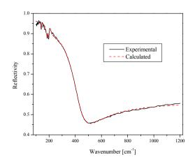
Fig. 1. Measured (solid line) and calculated (dash) infrared reflectivity spectra of PtSb<sub>2</sub>.
