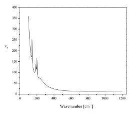
Fig. 2. Imaginary part of the complex dielectric function vs. wavenumber of PtSb<sub>2</sub>.
