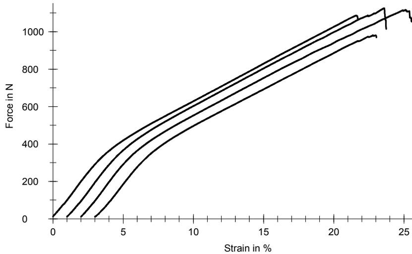
Figure 5. Force–strain diagram of the non thermo-stabilized sieve.
