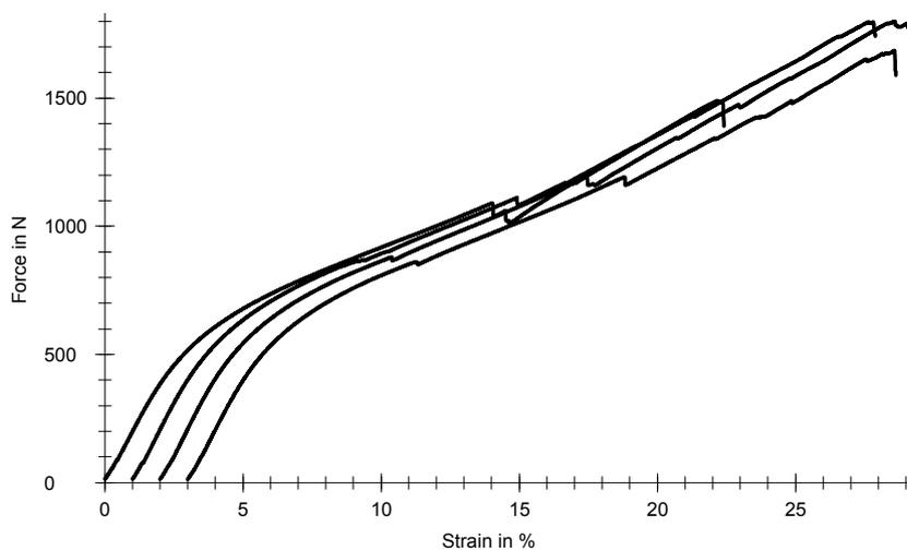
Figure 6. Force–strain diagram of the thermo-stabilized sieve.
