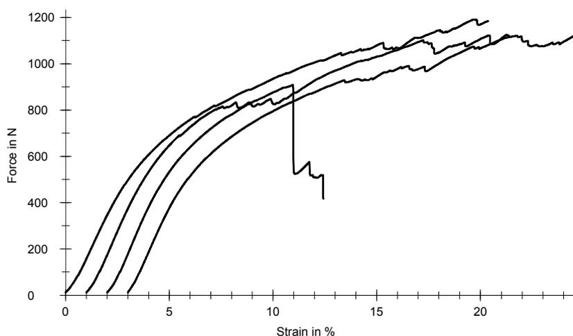
Figure 7. Force–strain diagram of the thermally stabilized sieve's joint.
