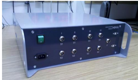
Figure 4. Two-bit quadruple three-phase power analyzer (MM4).
