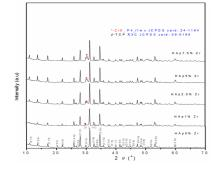
Thermal treatment of the prepared materials improved crystallinity and yielded to complete transformation of the initial apatite crystal phase into β-TCP, also important material in the field of hard tissue reconstruction.
