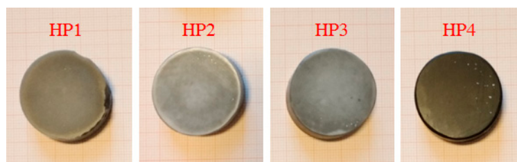
Figure 1. Sintered specimens: HP1—30 min-activated sample, HP2—nonactivated sample, HP3—30 min-activated sample with yttrium addition, and HP4—30 min-activated sample with graphene addition.
