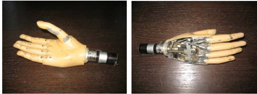
Fig. 3 The 'Belgrade hand'. The leverage mechanism that produces synergy of finger motions.
