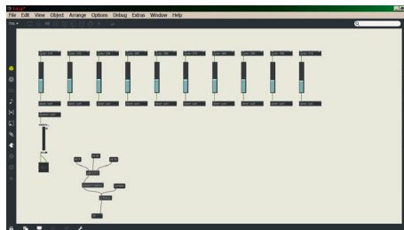
Figure 8: Work environment of the Max MSP software used for the synthesis of quantum sounds; this is a display of a patch that generates 10 harmonics
