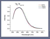
Photoluminescence emission spectra indicates wide greenyellow emission band with the maximum at 570 nm. This feature can be tentatively ascribed to the  ${}^{2}D{}^{-2}F_{5/2,7/2}$ electron transition of Ce<sup>3+</sup> ions in the YAG matrix.
