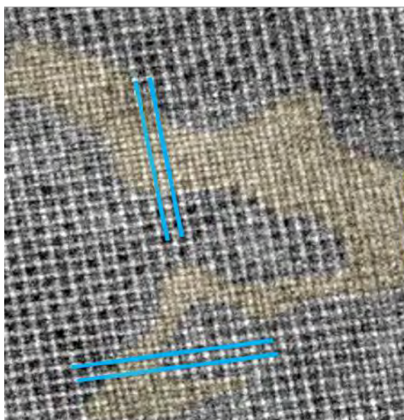
Figure 1. STEM LAADF image of FAPbI showing the coherent interface with PbI 2 precursor material and ordering of vacancies on the formamidinium sub-lattice. The unit cell size is 0.64 nm.
