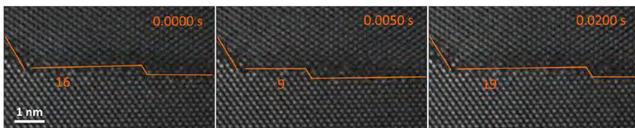
Figure 2. Sequence of images showing fluctuation of the step recorded with K2 camera at 217°C.
