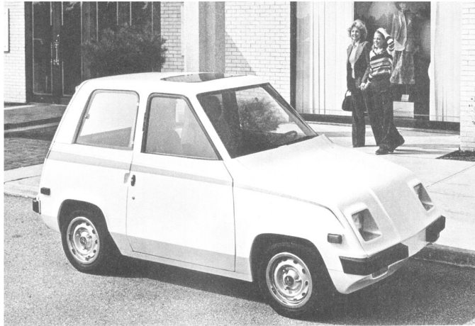
Figure 7. Copper City Electric Car Runabout power 15 kW made on the basis of cooperation for the use components of Renault R5.
