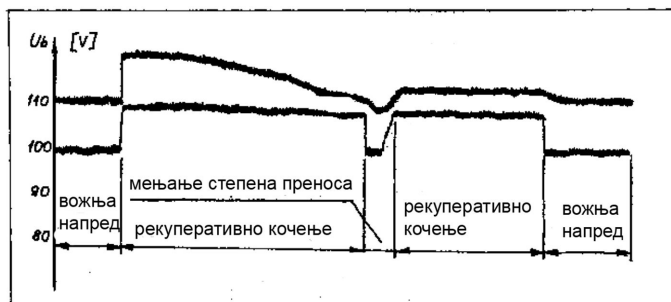
Figure 8. Change the battery voltage during DC recuperative braking in [15, 16].
