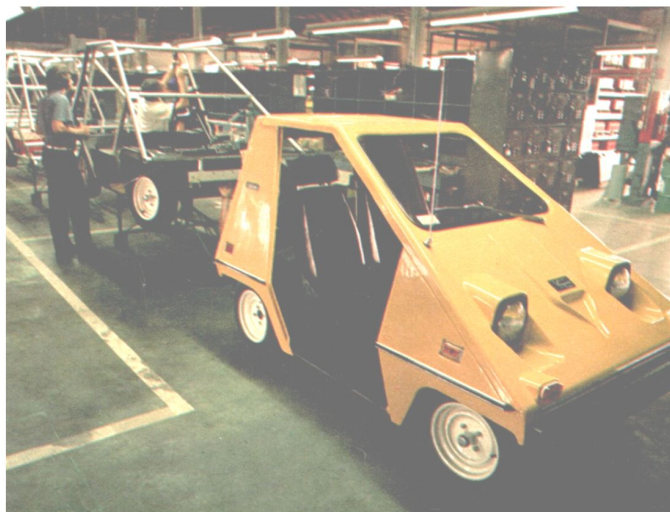
Figure 6. A typical city car (City Car) with two seats, weighs only 670 kg had a top speed of 28 mph (45 km/h) and radius of movement up to 65 km.
