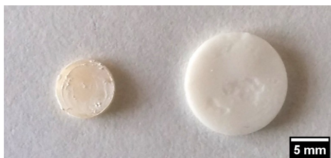
Fig. S.2. Photograph of the composite hydrogels synthesized using gamma irradiation (G-PLGA-PAA). Sample shown on the left is air-dried, and sample shown on the right is swollen to equilibrium in phosphate-buffered saline (pH = 7.4 and I = 0.154 M).
