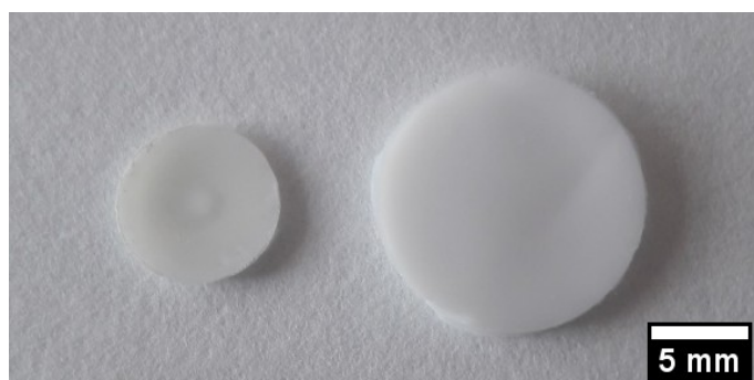
Fig. S.1. Photograph of the composite hydrogels synthesized using UV irradiation (UV-PLGA-PAA). Sample shown on the left is air-dried, and sample shown on the right is swollen to equilibrium in phosphate-buffered saline (pH = 7.4 and I = 0.154 M).
