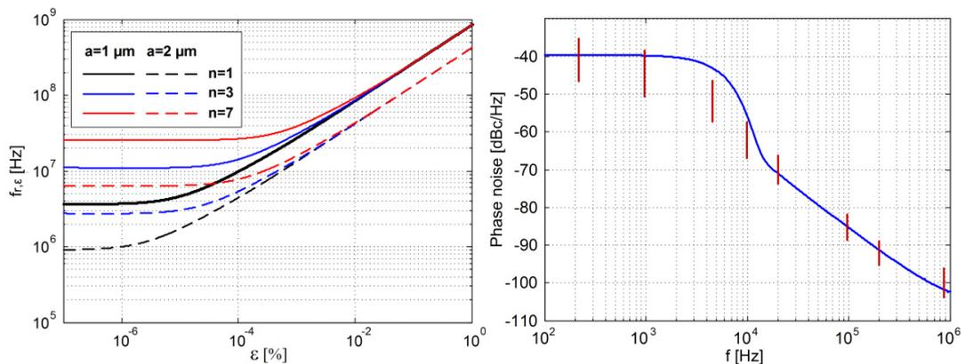
Fig. 2. (a) The graphene circular plate resonant frequency dependence on strain, for two different plate radii:  $a=1 \mu\text{m}$  (solid lines) or  $a=2 \mu\text{m}$  (dashed lines), and three different thicknesses, given by the number of atomic layers,  $n$ :  $n=1$  (black),  $n=3$  (blue) or  $n=7$  (red); (b) The oscillator phase noise obtained by numerical integration (blue solid line). The experimental data (Ref. [3]) are shown in red (discrete lines).
