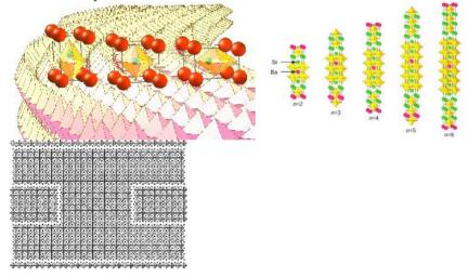
Strain engineering, dimensional confinement, epitaxial stabilization, and defect engineering applied to make today's best tunable dielectric even better in new  $(SrTiO_3)_{n-m}(BaTiO_3)_mSrO$  tunable dielectrics.
