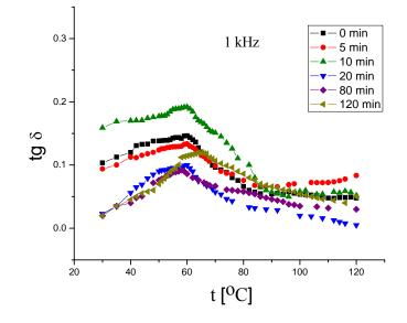
Fig. 6. Influence of activation time on the graph of temperature dependence of dielectric losses in BST sintered at v = 1 kHz.
