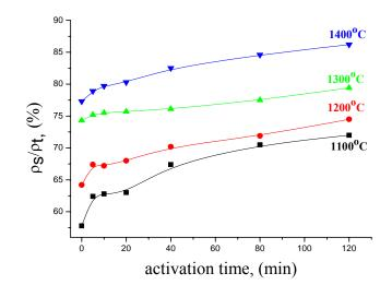
**Fig. 1.** Relative density in the dependence of activation time of BST-S sintered for 2 h at 1100, 1200, 1300 and 1400°C.
